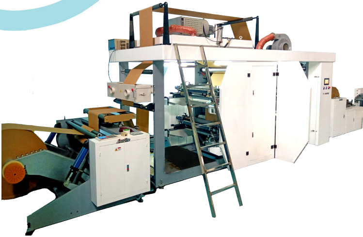
Roll-fed flexo printing Machine
